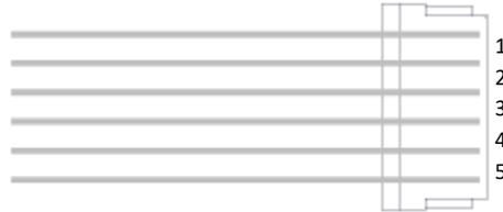
Fig 2. Pin configuration on the IM-21LQ000BD-2 module side of the 5-pin connector
