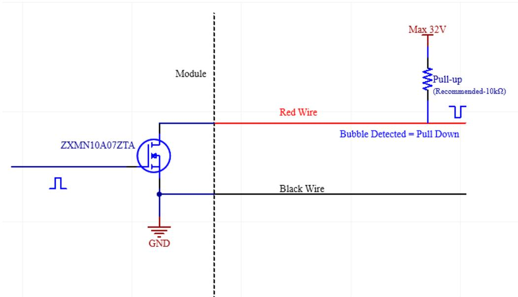
Fig 4. Simplified Schematic of Reference Measurement Circuit
